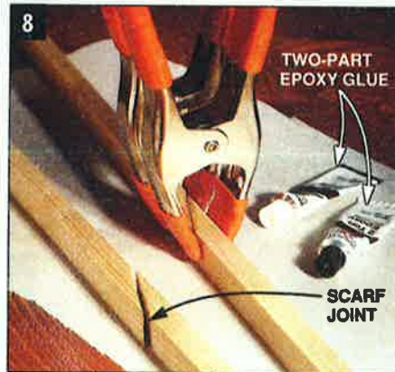
JOIN STRIPS of ash for the inwales and outwales with a "scarf joint," a low-angled lap joint. Glue the joint with epoxy.
