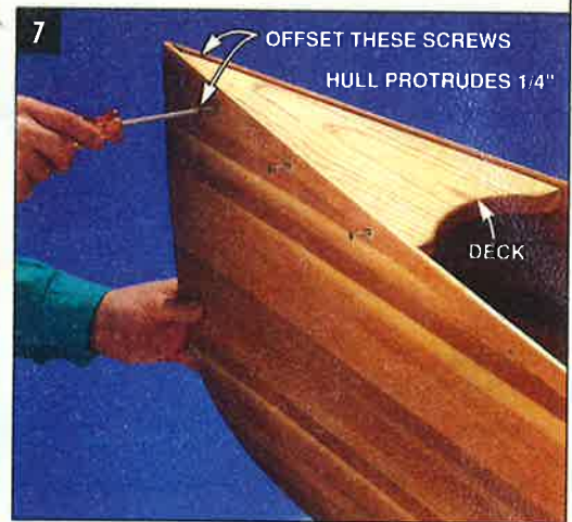
ATTACH THE ASH DECKS to the hull with stainless steel screws. Offset the two screws nearest the ends so they don't interfere with each other.
