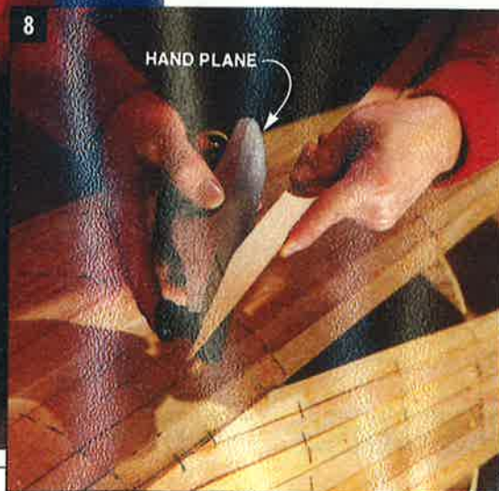
FILL IN THE BOTTOM of the canoe, working from the keel strip outward. A hand plane quickly cuts the tapered ends of the strips.
