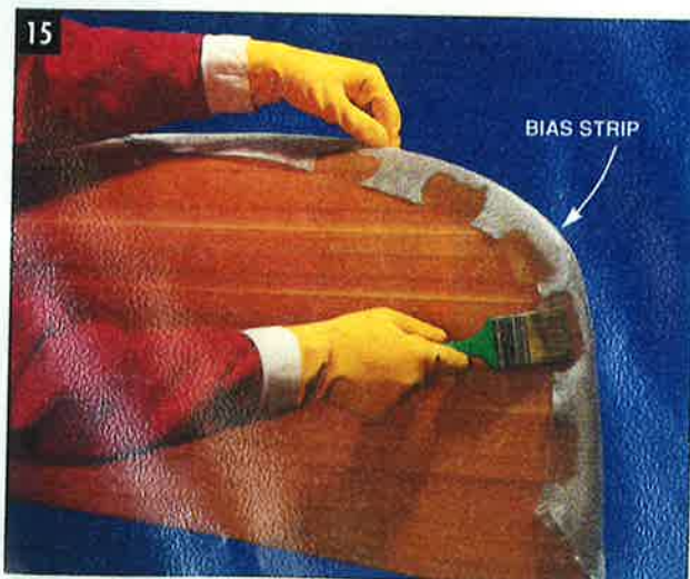
START WITH THE END STRIPS , laying down the dry cloth, then applying resin with a disposable brush. These strips (two under and one over the main cloth layer) provide extra strength in this critical area.
