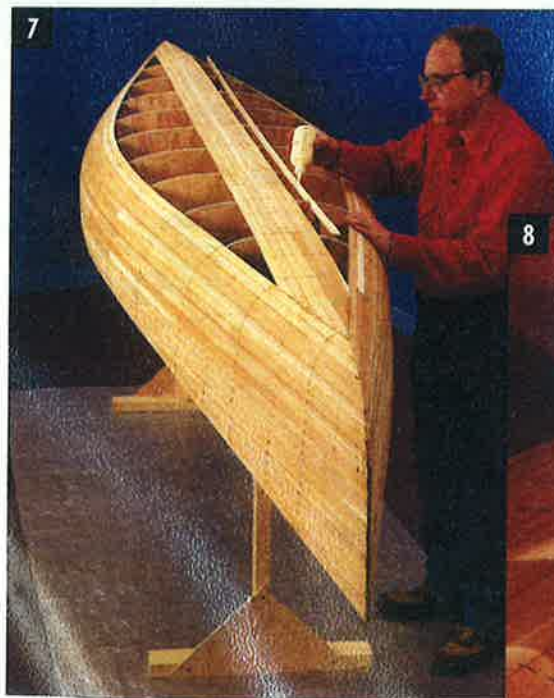
SPRING CLAMPS and slotted blocks help hold the strips in place where the molds are more curved. Between molds, short staples hold strips to each other.
