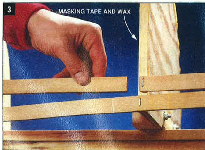
JOIN CEDAR STRIPS end-to-end, always putting the joint over a mold and keeping the joints spread randomly over the surface of the canoe.
