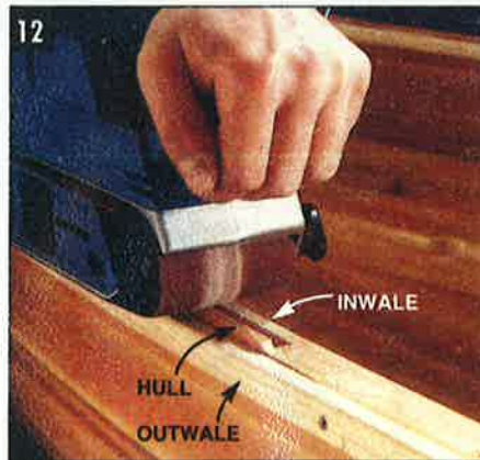
SAND THE GUNWALES FLUSH with a belt sander, removing the 1/4 in. of hull that protrudes. Hold the sander as flat as possible while you sand.
