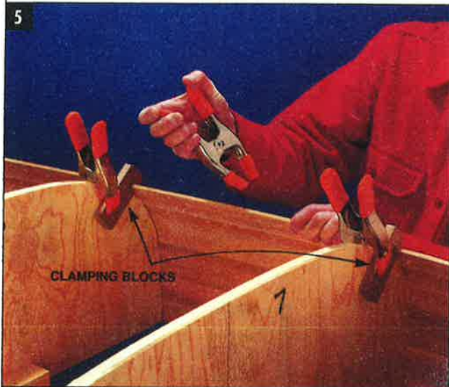
SPRING CLAMPS and slotted blocks help hold the strips in place where the molds are more curved. Between molds, short staples hold strips to each other.
