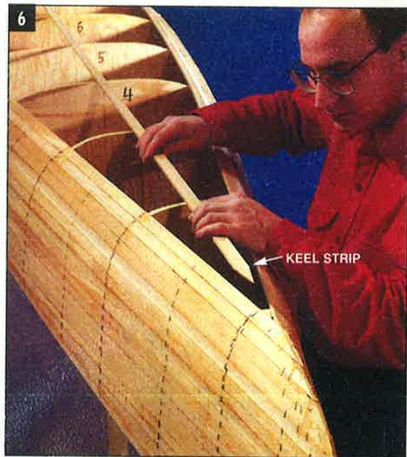
CUT THE KEEL STRIP to fit after all the horizontal strips are glued together. Staple the keel strip to the molds so it's exactly centered.
