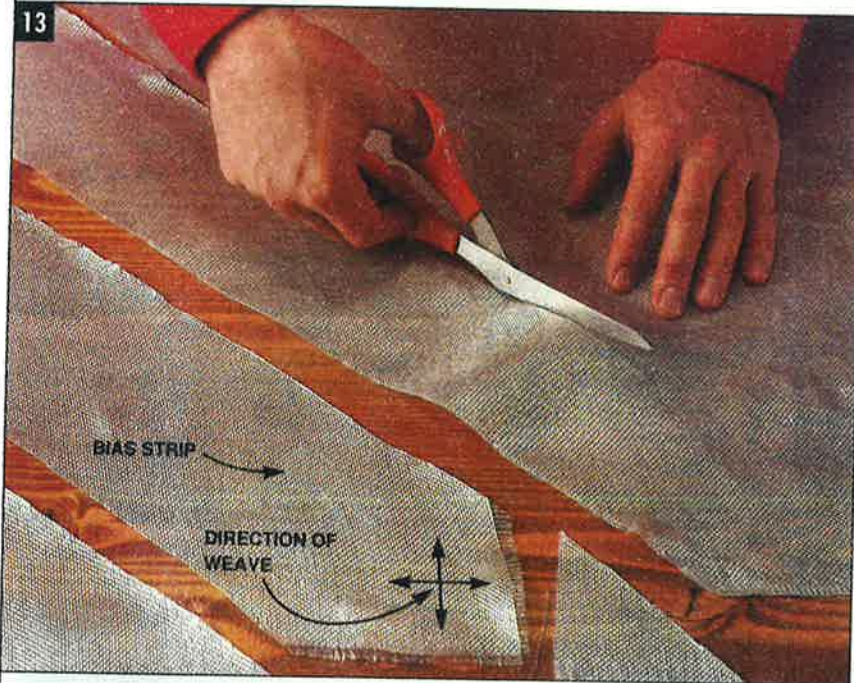
CUT STRIPS from the scraps to cover the ends of the canoe. Cut them at 45 degrees to the weave (on the bias) and make the ends pointed.
