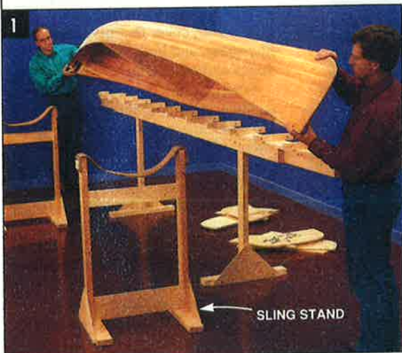
1 REMOVE THE CANOE from the strongback and place it on sling stands, which support it while you work on the inside of the hull and the trim.
