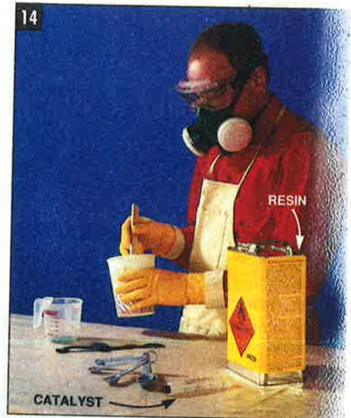
SAFETY FIRST! The resin that goes on the fiberglass cloth and its catalyst are both dangerous. Wear a carbon-filter respirator, goggles and rubber gloves.
