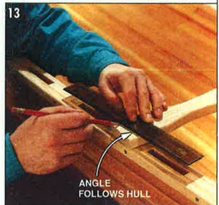
MARK THE THWARTS so they fit the angle of the hull, cut them, then bolt them on underneath the inwales with stainless steel bolts.
