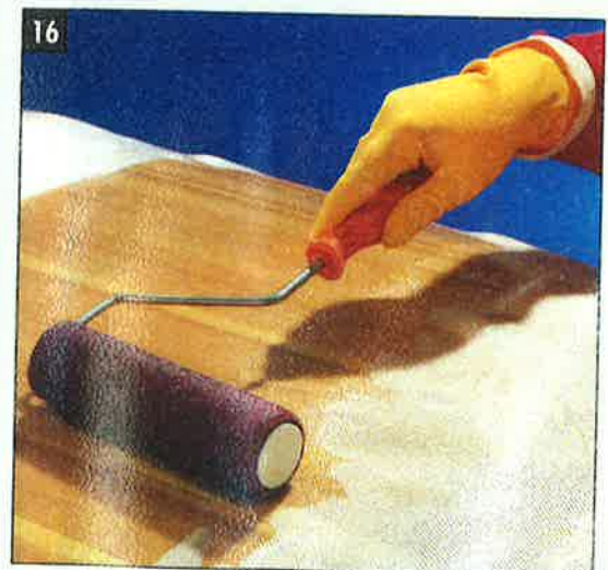
APPLY CLOTH AND RESIN to the entire hull. Lay the dry cloth on the hull, and apply the resin with a paint roller. Work out from the center in 2-ft. sections. Let it cure, sand and it's done.
