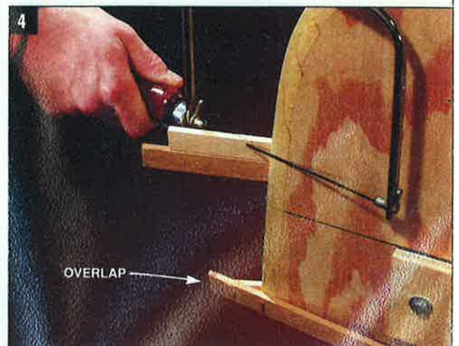
USE A COPING SAW to trim the ends of the strips. Note how the ends of strips on opposite sides of the canoe overlap. Temporarily laying a strip on the other side will allow you to mark the strips for cutting.
