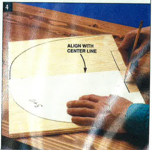
2 TRACE the shape of each mold to a separate sheet of tracing paper, taping it securely to the plywood layout board for accuracy.
