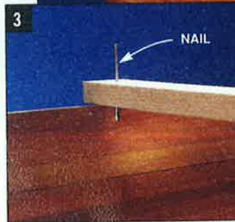
2 WOOD BRACES with nails at the ends keep the hull from bowing in when you're not working on it. Use the molds to determine the nail spacing.
