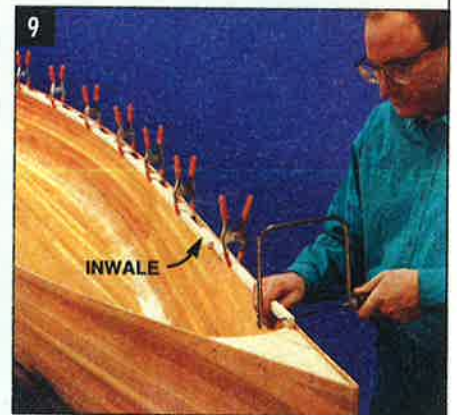
CLAMP THE ASH INWALE to the hull 1/4 in. below the edge, and trim one end to fit. Screw the inwale to the hull, then trim the other end.
